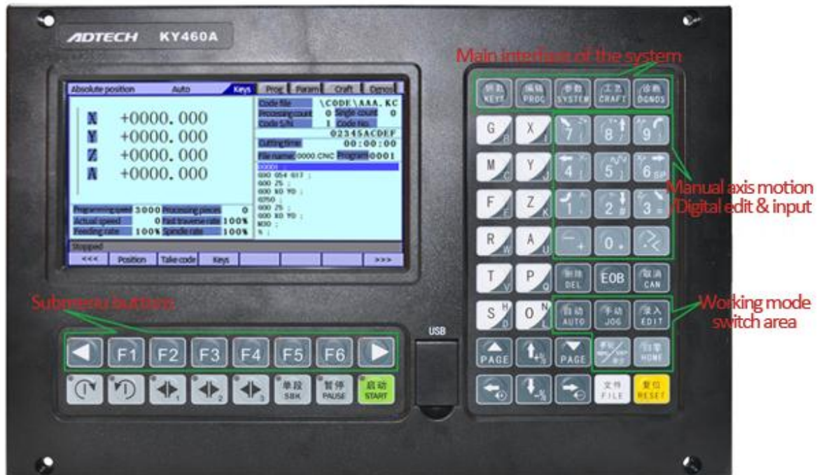
Fig. 3.1.1.1 Diagram of KYX60A series operation panel
